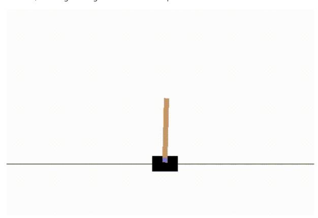
How it works is that a programmer sets some boundary conditions, and a reward function. The boundary conditions will be that the cart must stay within the boundary, and the pole must stay between say 75 and 105 degrees. The reward function will give points for the cart being closer to the middle, give points for the pole being closer to 90 degrees, and take points away if the cart goes too far towards the boundary or the pole moves away from 90 degrees.
